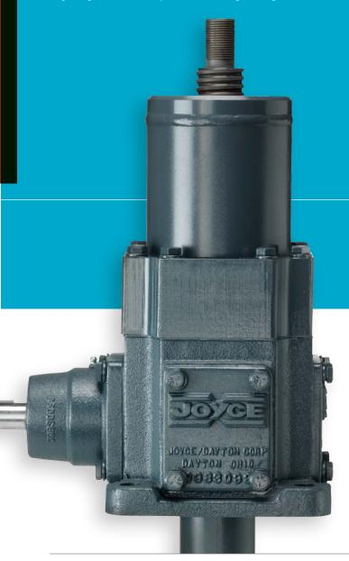
Joyce high-efficiency bevel ball actuators (BB) are designed for near-continuous duty operation. BB series actuators provide higher speeds and less heat generation than other mechanical actuators and require a brake motor or other external locking device to hold position. They also offer more precise positioning and repeatability than hydraulic cylinders.
