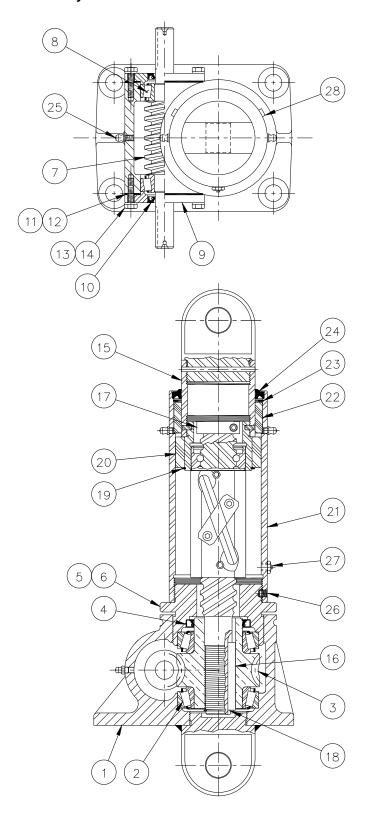
Table 3-2 Parts list – Ball Screw Electric Cylinder
