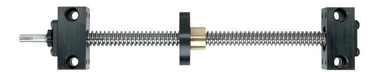
Joyce/Dayton offers Acme 2C and Stub Acme machine screw and nut assemblies in a variety of screw leads and in diameters ranging from ½ inch to 6 inches. Screws are typically made from alloy steel. Stainless steel material is available for many sizes. Most screws are available in both right-hand and left-hand thread directions, with corresponding bronze nuts and steel flanges. Screw stock is available in maximum lengths of 12 ft. and 24 ft., depending on screw diameters.
