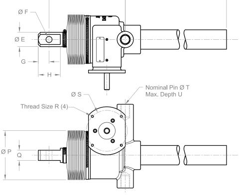
Trunnion pins should be made of steel with hardness greater than 30 HRC, yield strength greater than 110 KSI, and supported within 1/16 inch of the actuator housing.
