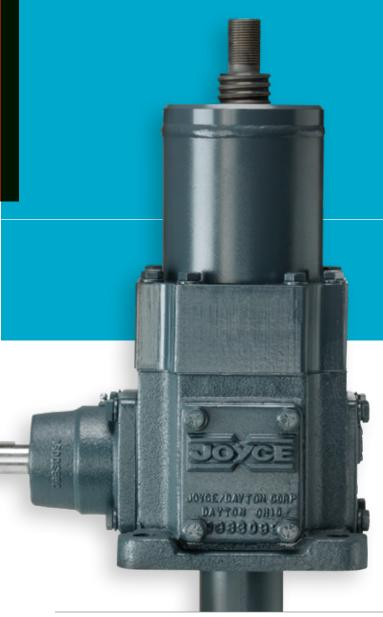
Joyce high-efficiency bevel ball actuators (BB) are designed for near-continuous duty operation. BB series actuators provide higher speeds and less heat generation than other mechanical actuators and require a brake motor or other external locking device to hold position. They also offer more precise positioning and repeatability than hydraulic cylinders.
