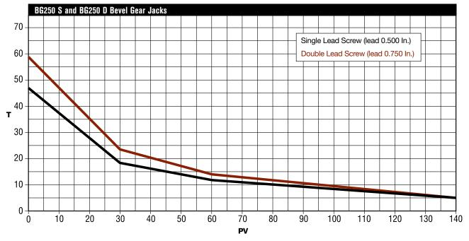
Note: PV =  $\frac{\text{load x velocity (fpm)}}{1000}$
