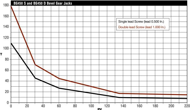
Note: PV =  $\frac{\text{load x velocity (fpm)}}{1000}$
