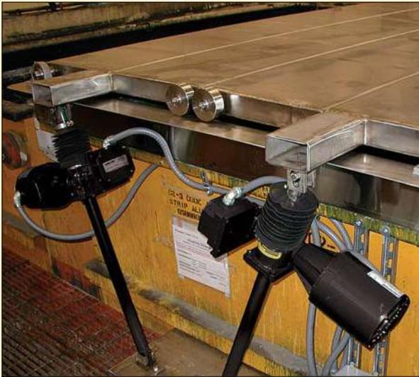
When engineers needed a quick and compact way of opening the large doors of these plating tanks, they selected a UNI-LIFT solution. The application utilizes two 5-ton double-clevis Screw Jacks, with a motor and a limit switch box mounted on each. The operator just pushes a button to open the doors and pushes another to close them. This method greatly enhances operator safety and helps prevent cross-contamination between tanks.
