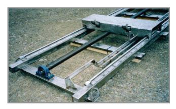
As the ComDRIVE powers the transfer system, nuclear waste is conveyed down a 80-foot long corridor. As the load traverses it is transferred across thresholds onto successive ComDRIVE systems until it travels the full distance. Stainless steel doors close as it passes each threshold sealing the nuclear waste in an inner chamber.
